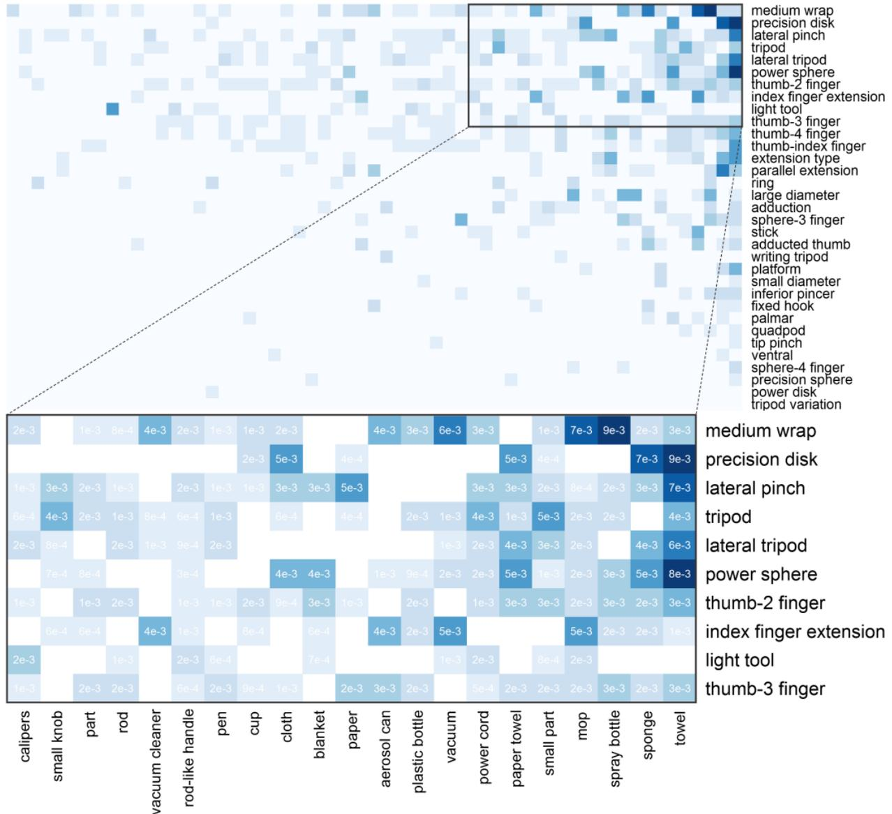
Fig. 3. Normalized grasp-object matrix,  $M$ , which shows how strongly each grasp is associated with each object. The top shows the entire matrix, and the bottom shows a zoomed in portion for the most common grasps and objects. The value in each cell is normalized to represent the proportion of the data in the entire matrix. For example, the upper right cell shows that the medium wrap used with the towel object is 0.3% of the total grasp-object matrix data.
